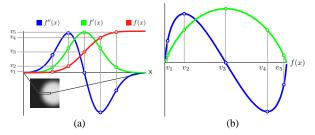
Figure 4: The behavior of primary data value (f), gradient magnitude (f'), and the second directional derivative (f'') as a function of position (a) and as a function of data value (b).
